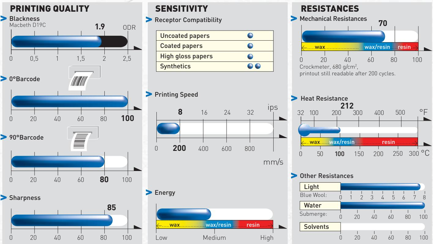
Evaluation of observed performances of the ribbon with optimised printer, settings and receptors (ARMOR procedure).
